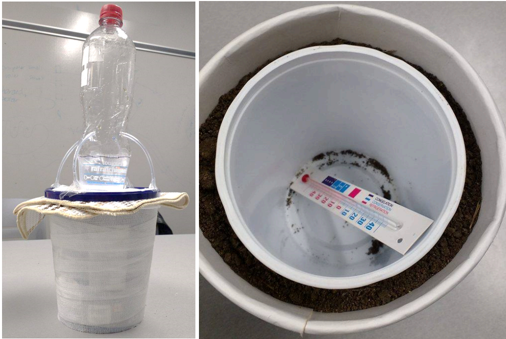
Figure 9: Pictures of proof-of-concept prototype that was built. Right: View of soil layer. Left: View of entire fridge system.
